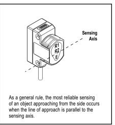
Figure 2. Fixed-field sensing axis
