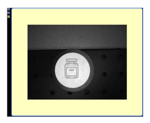
Note: The reference image is used as a template for developing an inspection; it establishes the initial values for the Vision tools. The reference image also is used by Quick Teach.
