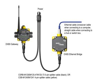
Connect a DX83 Ethernet Bridge to a host system using the industrial Ethernet connection on the DX83. To connect the DX83 directly to the host system without using an Ethernet switchbox/hub, some host systems may require a crossover cable.
