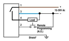
\* It is recommended that the shield wire be connected to either earth ground or DC common.
