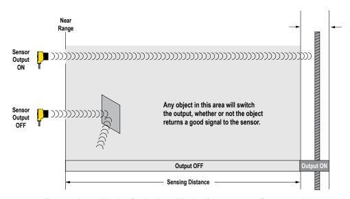
Figure 5. An application for the Auto-Window feature (retroreflective mode)
