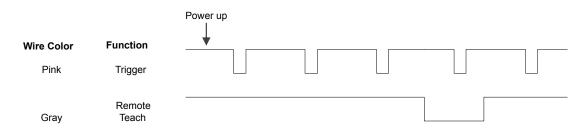
The sensor triggers from high to low, and Remote Teach behaves electrically like trigger.
