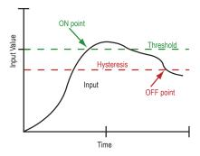
In the example shown graphically, the input is considered on at 15 mA. To consider the input off at 13 mA, set the hysteresis to 2 mA. The input will be considered off when the value is 2 mA less than the threshold.
