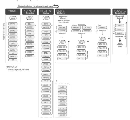
From the \*RUN Menu (or any menu), single-click button 1 to advance through the top-level menus. Top-level menus are displayed on the LCD with an asterisk (\*) in front of the menu name.
