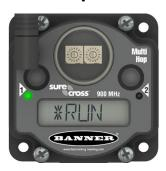
When power is applied, the MultiHop radio begins running. The display screen autoscrolls through the \*RUN menu and communication between the devices is enabled. Autoscrolling through the \*RUN menu is the normal operating mode for all devices on the wireless network.
