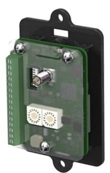
SureCross® Performance embeddable board modules were specifically designed for the needs of industrial users to provide connectivity where traditional wired connections are not possible or cost prohibitive. Wireless networks are formed around a Gateway, which acts as the wireless network master device, and one or more Nodes. SureCross Performance embeddable board modules communicate with all SureCross Performance radios.
