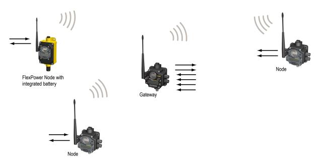
The SureCross® Performance network is a deterministic system—the network identifies when the radio signal is lost and drives relevant outputs to user-defined conditions. Once the radio signal is reacquired, the network returns to normal operation.
