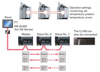
NS/NT-series PTs can also be incorporated as slaves (1:N NT Link connections) to exchange data using the NT Links with only the master CP1H. Each is treated as one slave node
