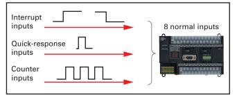
The 8 normal inputs (6 for Y CPU Units) can be selected in the PLC Setup as interrupt, quick-response, or counter inputs.
