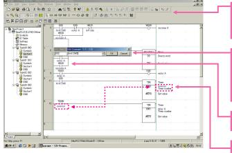
Shortcut keys can be easily checked using the ladder key guide. Programming is simplified by key inputs, such as the **C** Key for an NC input (contact), the **O** Key for an OUT instruction, and the **1** Key for special instructions.
