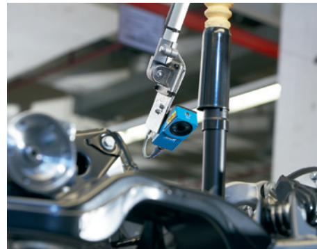
Verification of hole presence as well as nuts, safety springs and washers
