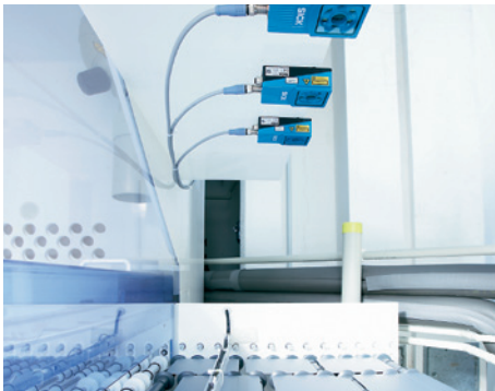
Verification of part assembly before next station
