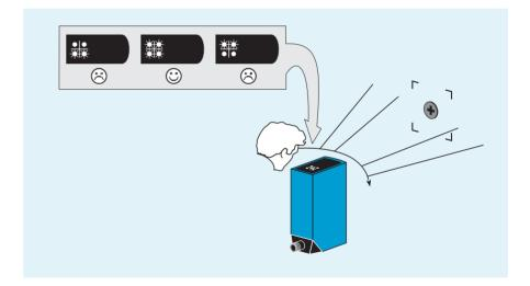
No special settings or programming of the DMP is required. The DMP Position Finder must only be aimed at the reflector, and then it is ready to operate. When operation of the DMP is started, all four control lamps light for a brief time (→ function test).
