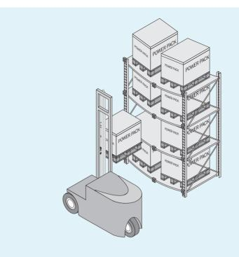
${\color{blue} \blacktriangle}$  Differing location measurements caused by weight do not affect the accurate positioning procedure when the DMP is used.
